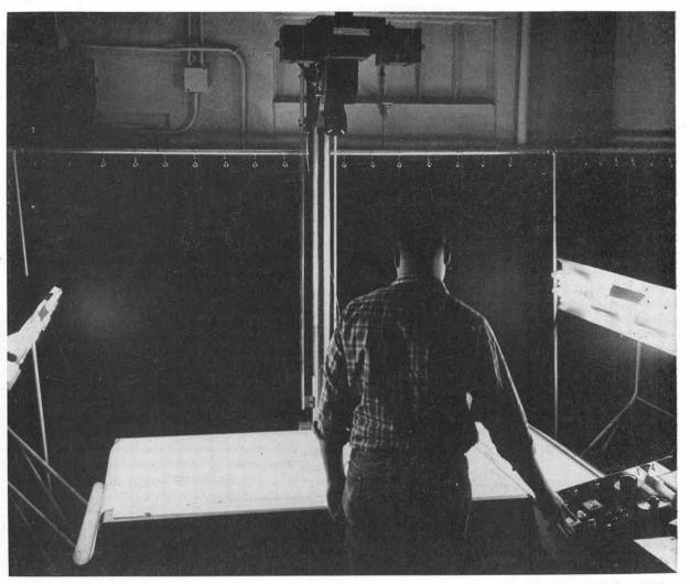
NEW PHOTO DEVICE CAMERA, operated by Don Fulton, has improved quality of prints. About 1600 exposures are taken daily on this camera. Drawings are reduced on 35mm film 16 to 30 times depending on the size of the drawing. Prints which will be sent to suppliers are made from the 35mm negative mounted on an IBM card by Diazo Reproduction Section 3462-2 on a Copy Flow machine.
